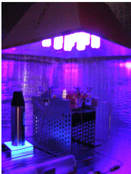
Figure 1: Photo showing sample chamber (center) with Peltier-cooler during irradiation by UV lamp (top). To the left the photo-spectrometer is visible.
